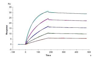
Human IL-17R alpha, hFc Tag captured on CM5 Chip via protein A can bind Biotinylated Human IL-17A, His-Avi Tag with an affinity constant of 2.18 nM as determined in SPR assay (Biacore T200).
